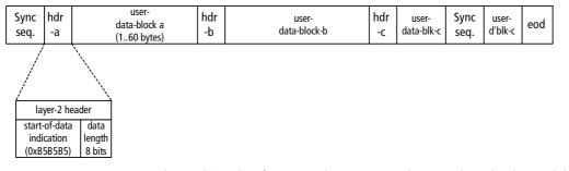
The eod (End Of Data) indication merely provides a lead-out delay to ensure that the data is completely sent before the transmitter is turned off.
