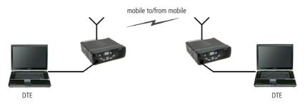
In this configuration the DTE is connected to the TM8000 via the serial port, data is sent from DTE to DTE via the TM8000 radio modems.
