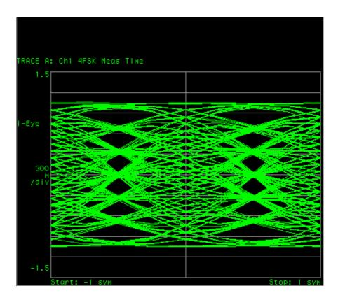
Like C4FM, this is a four-level FSK scheme, but can achieve higher data rates while maintaining compliance with ETS300-113 ACP. This scheme is a form of minimum shift keying, and hence is a subset of MSK.
